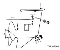
Put a new gasket on the oil level plug.
